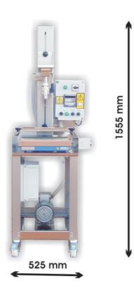
AISI 304 stainless steel frame This filling machine works by weight Suitable for liquids not charged with gas and stiff containers Maximum weight: 5 Kg Filling through a flexible impeller pump The product weight is set through a display Self-zeroing of the tare on starting The filling speed is adjustable
